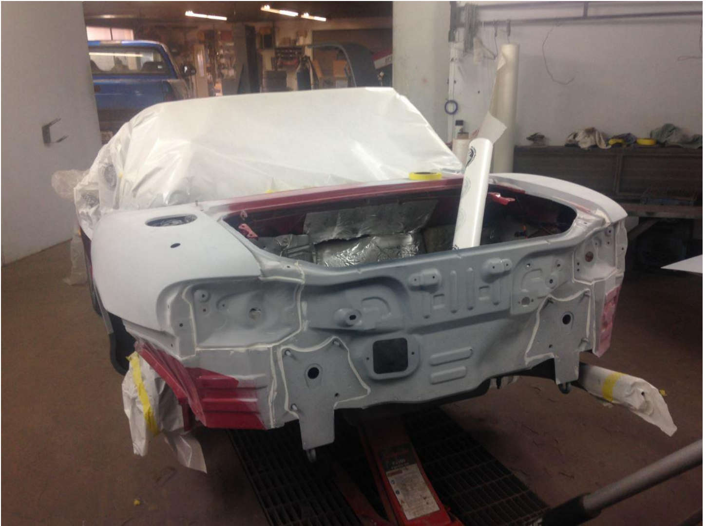
Trunk lid and bumper cover epoxy primed and ready for blocking to prepare for painting Oct 26 th 2017.
