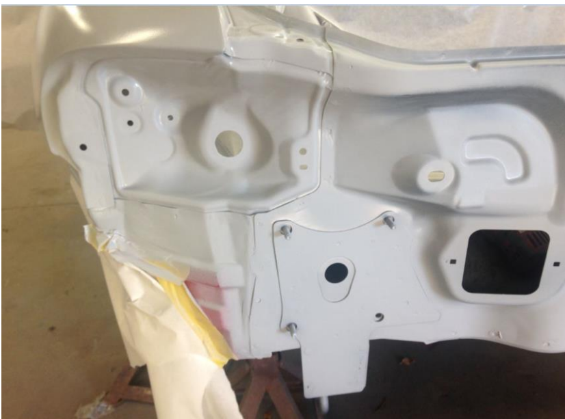
Detail photos of the left and right rear panel areas. The square opening is for the air release flap. New pone of those was needed too.
