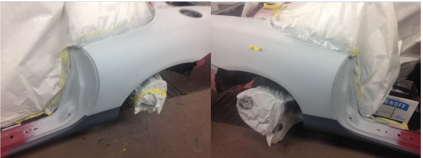
Rocker guard applied to new rear quarters - Oct 26 th 2017.
