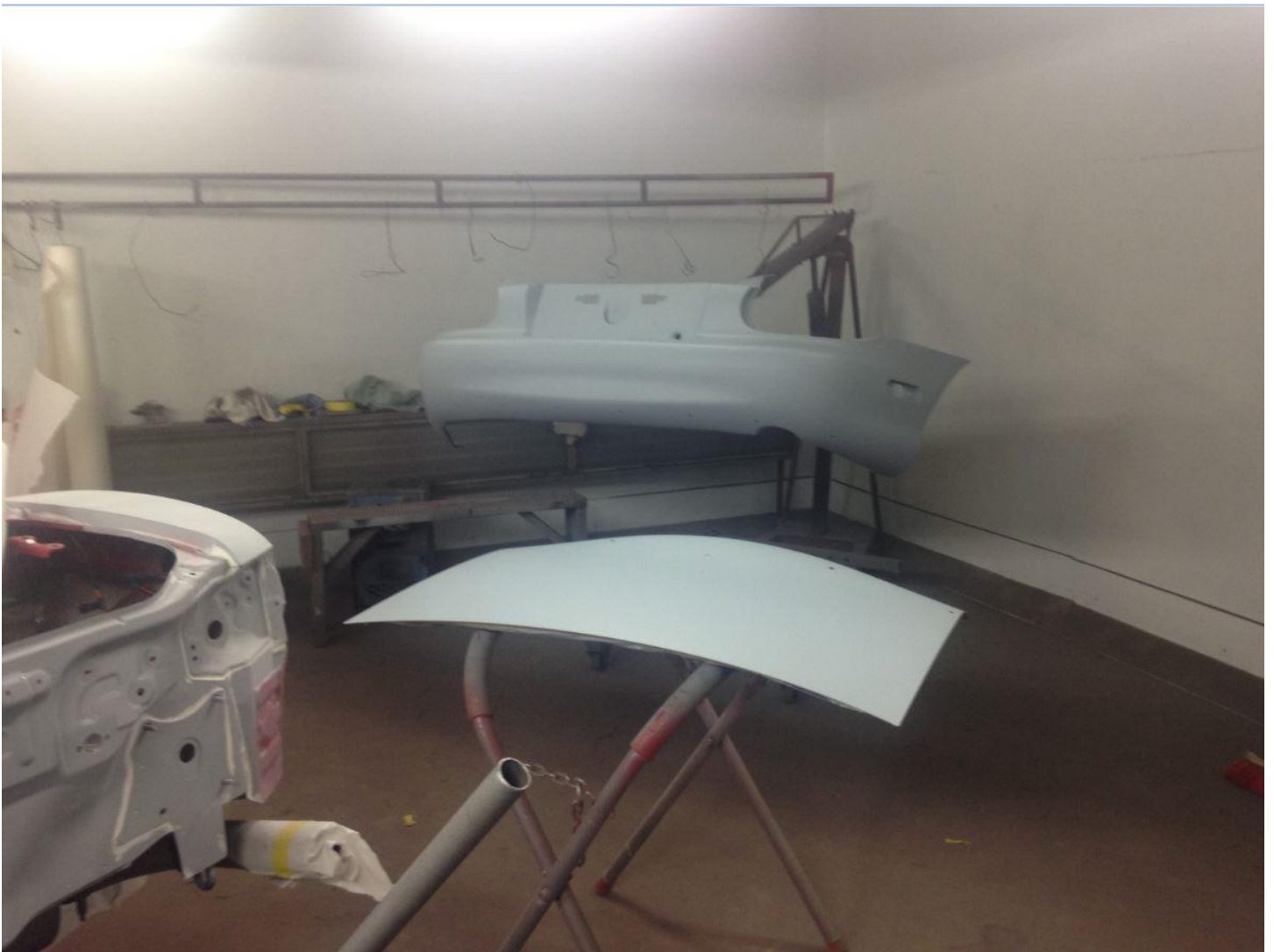
Trunk lid and bumper cover epoxy primed and ready for blocking to prepare for painting Oct 26 th 2017.
